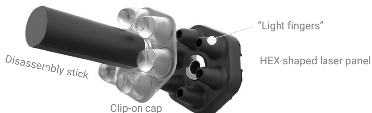
Graphic 14: Replacement of a protection cap with the magnetic stick
